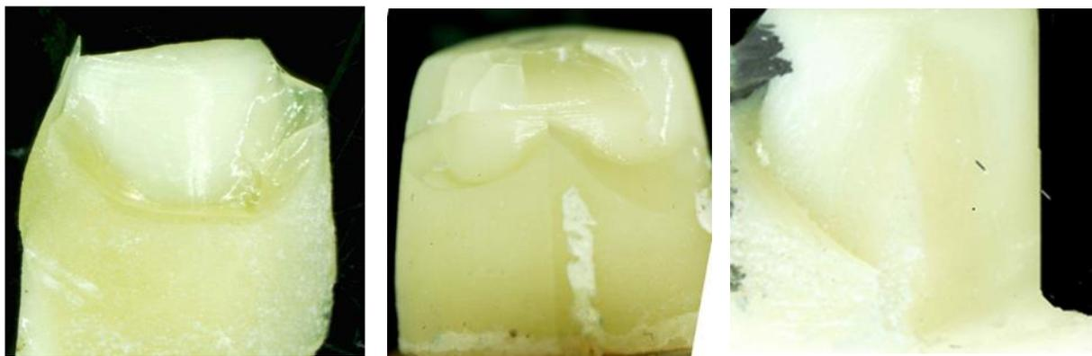
**Fig. 3:** External surface of a fractured specimen with a modified core (MC) design at  $\times 10$  magnification
