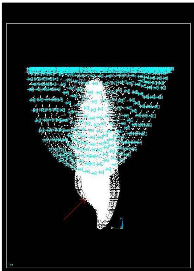
**Fig. 3:** A 100-N compressive load was applied to a load-bearing area of 1 mm<sup>2</sup> on the lingual surface of the tooth
