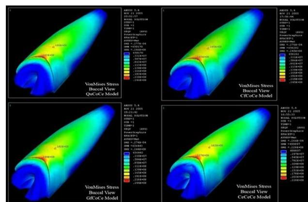
**Fig. 6:** Maximum von Mises stress (VMS) in quartz fiber post (QuCoCe), carbon fiber post (CfCoCe), glass fiber post (GfCoCe), and zirconia post-and-core (CeCeCe) restored with all-ceramic restorations (ACRs)
