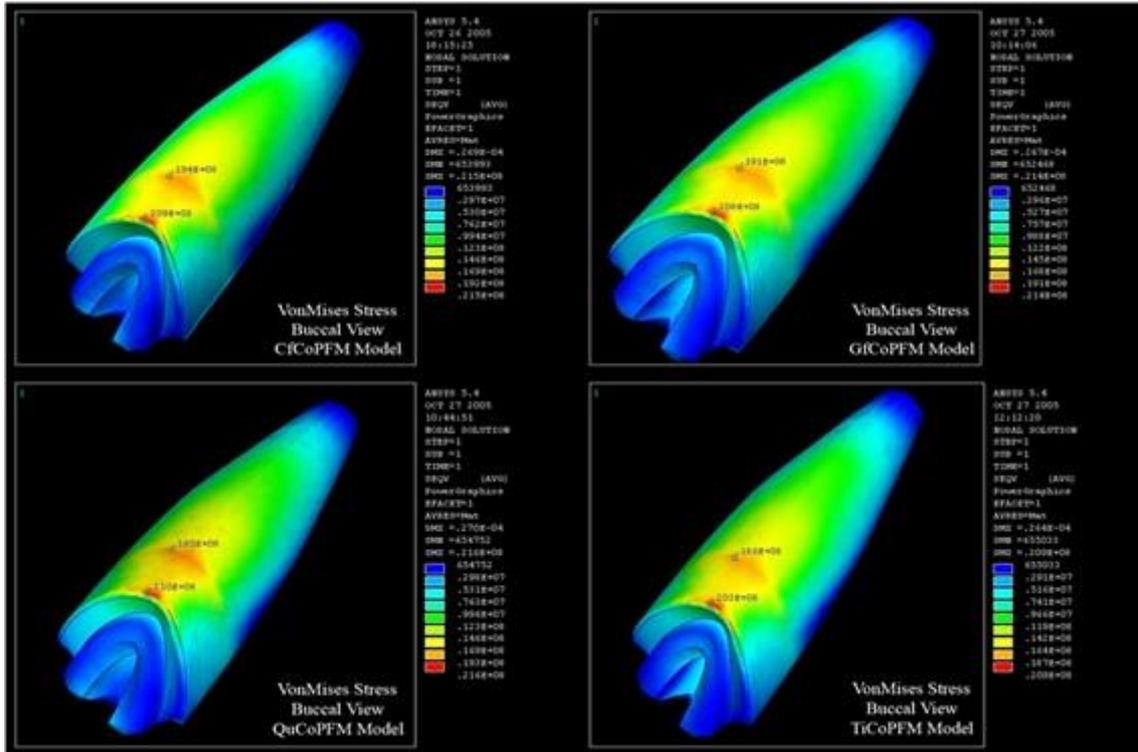
**Fig. 5:** Maximum von Mises stress (VMS) in carbon fiber post (CfCoMCR), glass fiber post (GfCoMCR), quartz fiber post (QuCoMCR), and titanium post (TiCoMCR) with composite cores and metal-ceramic restorations (MCRs)
