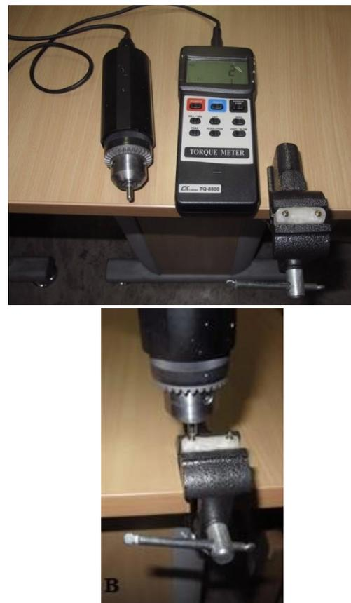
**Fig. 6:** The electronic-torque-meter (A) is tightening the abutments (B)
