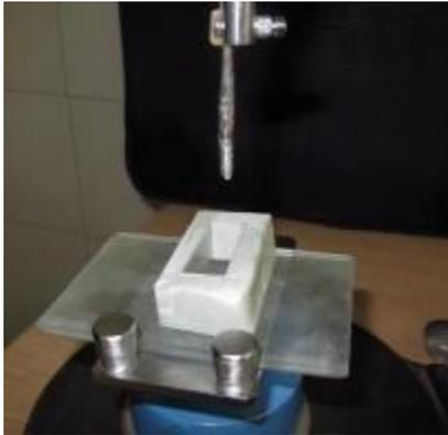
**Fig. 3:** Insertion of implants by using the surveyor
