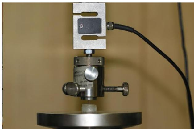
Fig. 3: Push-out test
