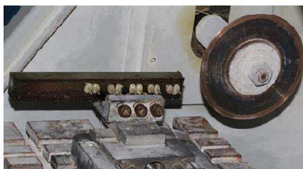
Fig. 2: Sectioning of the mounted samples
