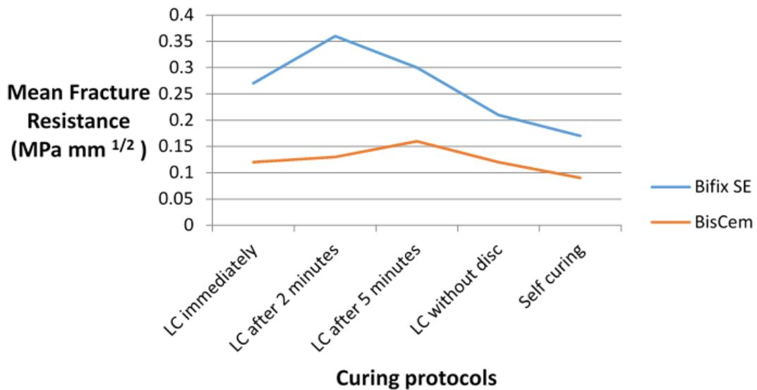
Fig. 5. Mean fracture resistance (K<sub>IC</sub>; MPa/mm<sup>2</sup>) of the two cement types according to the curing protocols, LC=light-curing
