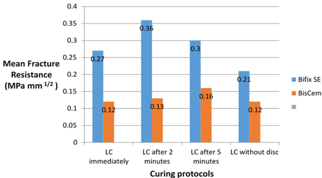
Fig. 6. Mean fracture resistance (K<sub>IC</sub>; MPa/mm<sup>2</sup>) of the two cement types according to the curing protocols, LC=light-curing
