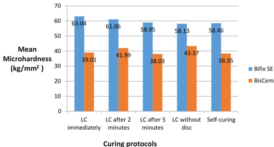
Fig. 4. Mean microhardness (Kg/mm<sup>2</sup>) of the two cement types according to the curing protocols, LC=light-curing
