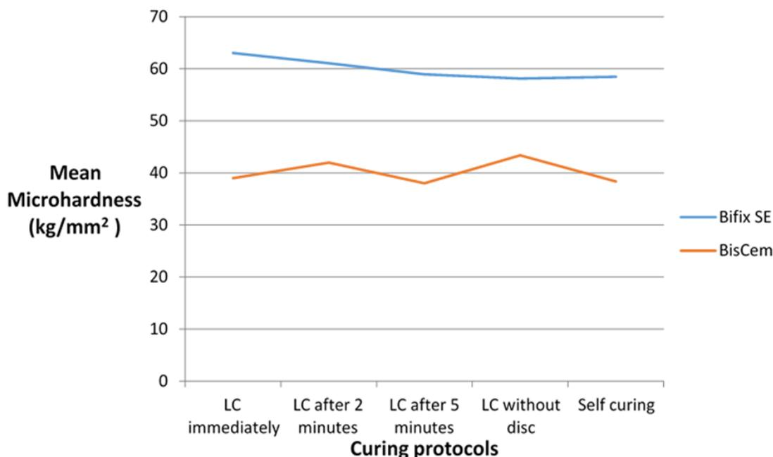
**Fig. 3.** Mean microhardness (Kg/mm<sup>2</sup>) of the two cement types according to the curing protocols, LC=light-curing
