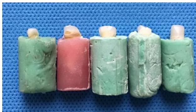
**Fig. 3.** Repairable fracture (above the CEJ)
