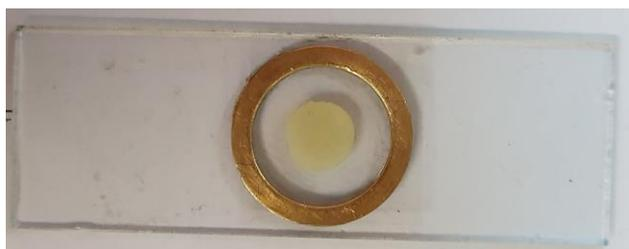
**Fig. 1:** A sample of a packed composite resin
